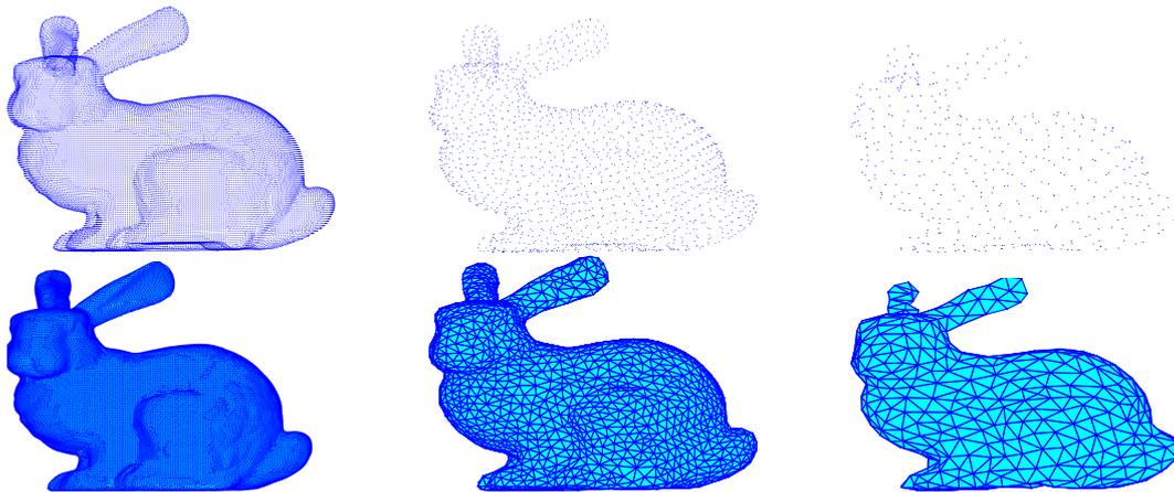
Figure 1: Point cloud sparsification of the 3D Stanford bunny model (top) and resulting triangulations (bottom).
